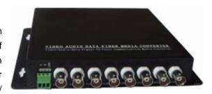
binary input/output over one multimode or single-mode optical fiber. These multiplexers are typically used in applications where the cameras have P/T/Z capabilities. Plug and Play design ensures the ease of installation and operation. Electronic and optical adjustments are never required. LED indicators are provided for instantly monitoring system status. Devices are available for either standalone or rack-mount installation, which is suitable for different working environment.
