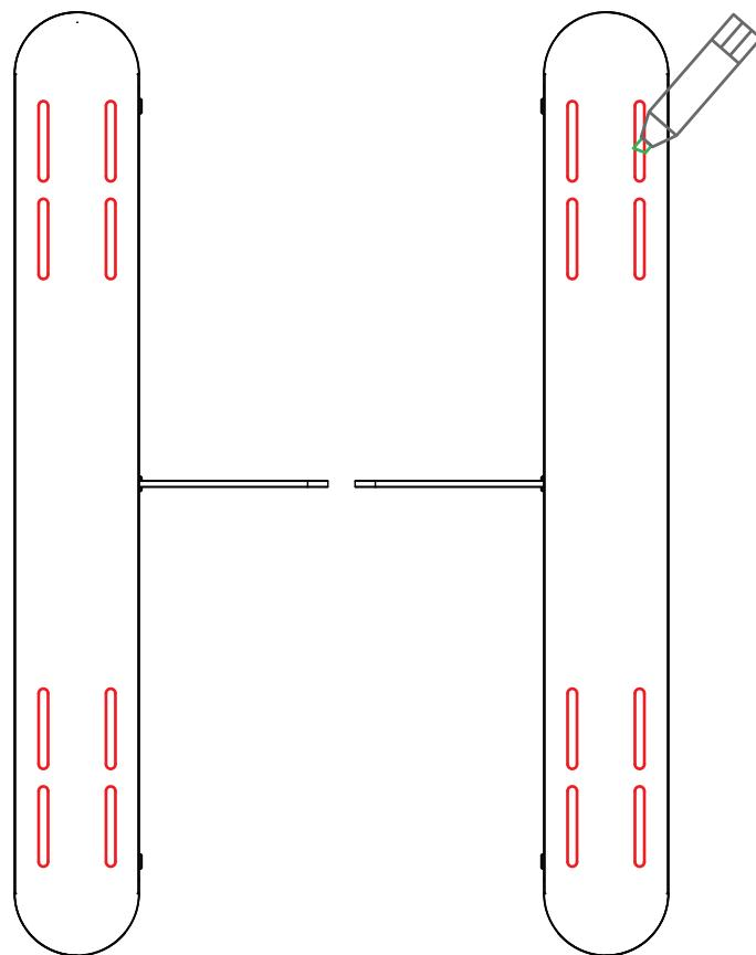
Move the device away and embed M12x100mm expansion screws according to the marked hole positions
