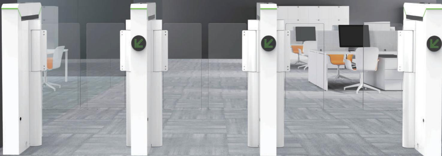
Mars-S100 series is ZKTeco's compact swing barrier turnstile, it is made of SPCC metal material and powder coating finishing. The length of cabinet of turnstile 600mm. This series including single and dual wing available. It is easy extension for multi-lane, wider lane ( 900mm ) as optional. It designed for smooth&silent operation and draws very little power also.
