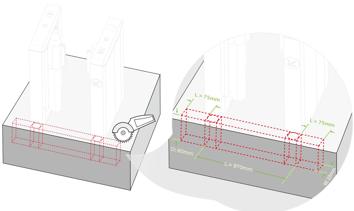
6. Clean up the debris and dust after drilling, and then place the turnstile back on the installation site. Check if the drilled holes align with the mark on the turnstile.
