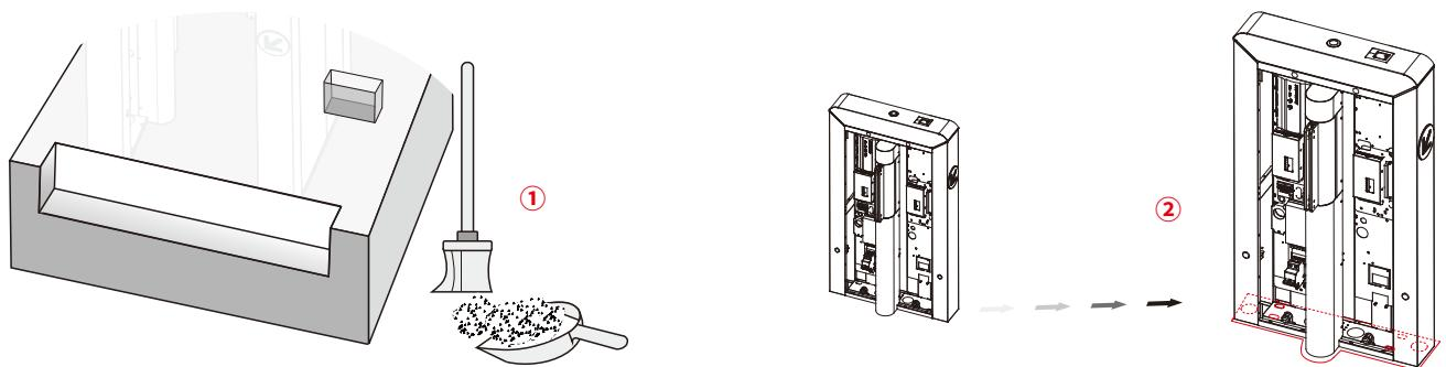
7. Put  $\Phi$  20mm PVC pipes, and insert Ethernet, Tether Cable and Power Cable through the pipe lines, and then pour the concrete to fill the conduit. **Note:** The strong and weak powers shall be laid separately.
