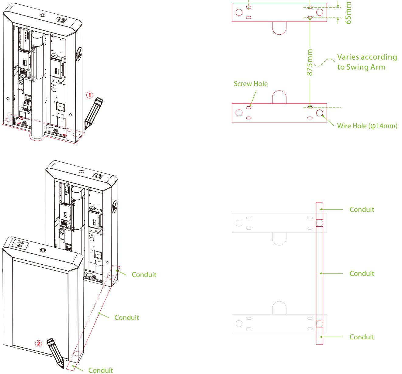
4. Remove the turnstile and use an electric drill to drill holes according to the markings.
