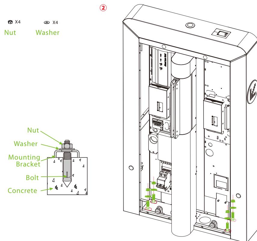
**Note:** Before inserting the bolt, the user must disconnect the power and Ethernet cables from the machines and place them into the conduit.
