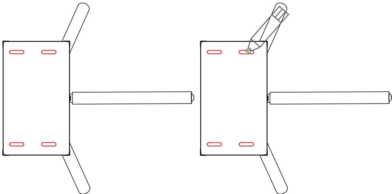
Move the device away and embed M12x100mm expansion screws according to the marked hole positions
