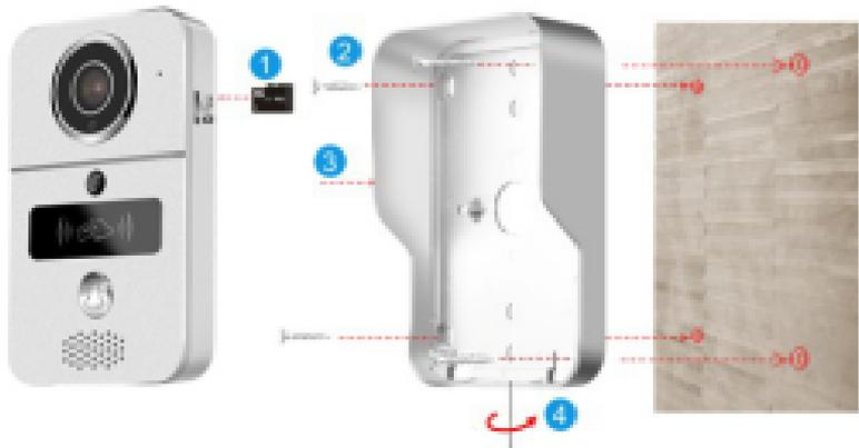
2 Use four screws in the four corners to fixed doorbell on the wall.
