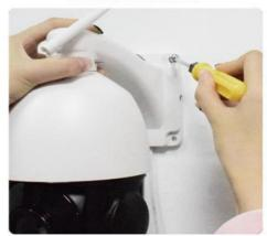
3. Align the screw hole on the bottom of the camera bracket with the hole on the wall. Screw in the screw to fix the camera.
